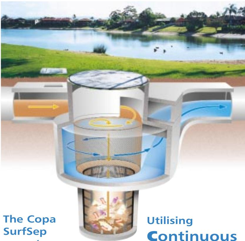
The Copa SurfSep operates continuously at any flow providing non blinding screening to 3mm in two dimensions.
