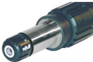
pH electrode, item no. 160310, 1 - 14 pH, 10 - 80 °C, 0 = 4.6 pH.
